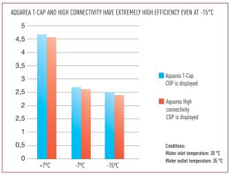
Aquarea T-cap always has high efficiency and high heating capacity even at extremely low temperatures. With Aquarea T-Cap, you can always enjoy high savings.
